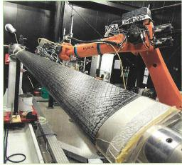
In situ production of a Krueger flap with an automated TP process
