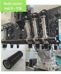
Inline monitoring sensor for draping processes
