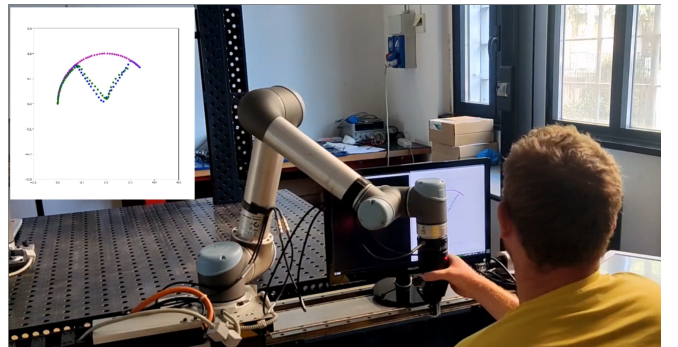
Fig. 1: The experimental setup, showing the application and the monitor displaying the three trajectories: magenta - robot desired trajectory, blue - human desired trajectory, green - actual trajectory.
